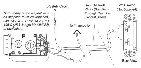
Figure 14 - Wall Switch Wiring Diagram
